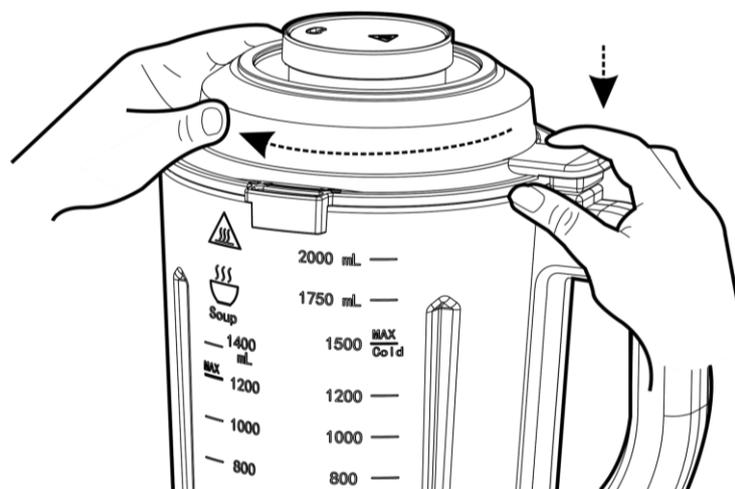
Figure 9 – Large lid closing procedure
